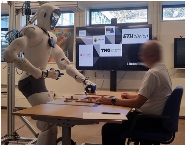
Fig. 3. Interaction between someone in the remote environment and the user present through the telepresence robot. They are working together to complete puzzle.
