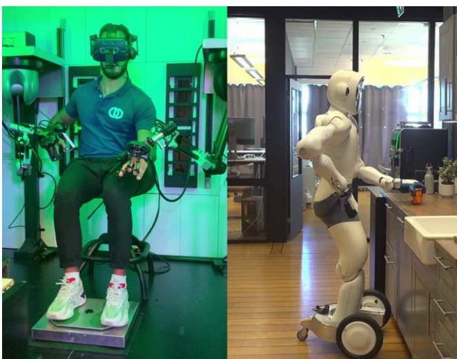
Fig. 2. The user inside the pod (left panel) controlling the humanoid telepresence robot on the right in a kitchen 800 km away.
